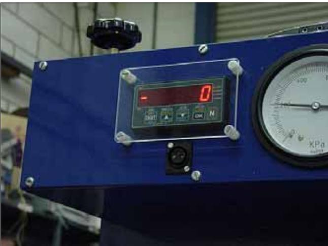
A digital display readout on the machine's front panel allows the operator to see the load currently being exerted, the operator can then use this display to more accurately set the required load for grading in Newton's instead of Kpa.
