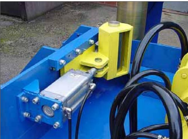
A heavy duty output drive roller is used to ensure timber is driven out of the machine after the grading process, the output drive also ensures that the timber is presented correctly to the roller markers during the final grade marking.
