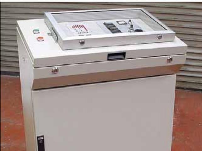
The controls are cover by a transparent lockable hood, which whilst keeping the control panels free from dust and other debris, still allows the operator to monitor the status of the machine.
