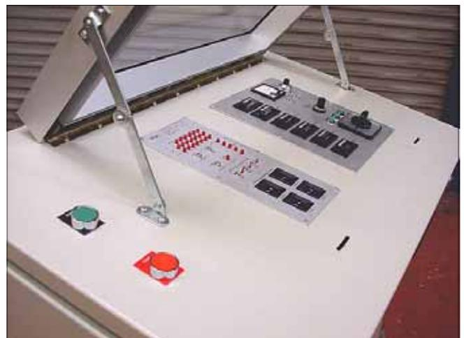
The console connects to the grading machine via two 36-way connecting leads, these two leads carry all the signals required to run the machine. The standard length is of these is 5 metres.
