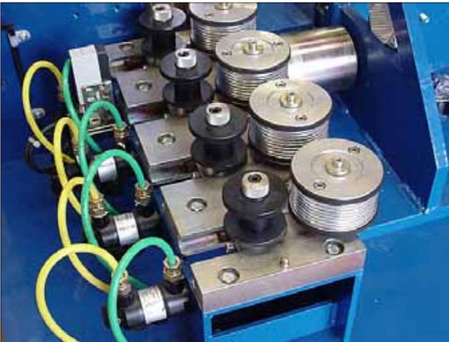
All pneumatic control valves and operating solenoids are collectively mounted in a separate panel this allows ease of access during any servicing.
